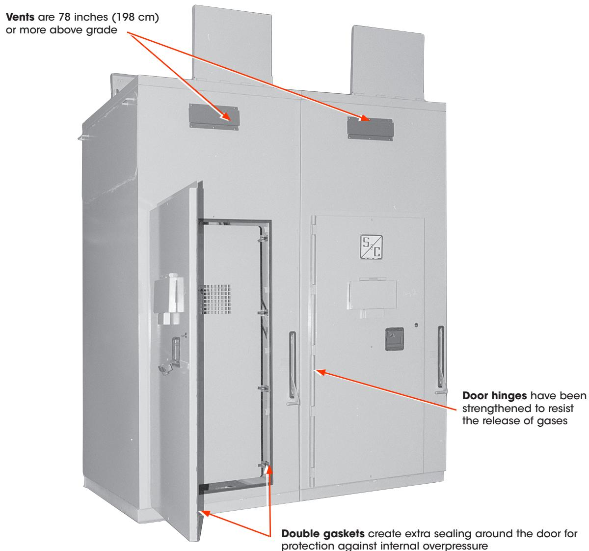
Figure 1. Front view of top-flap style arc-resistant S&C Metal-Enclosed Switchgear rated 25 kV.
