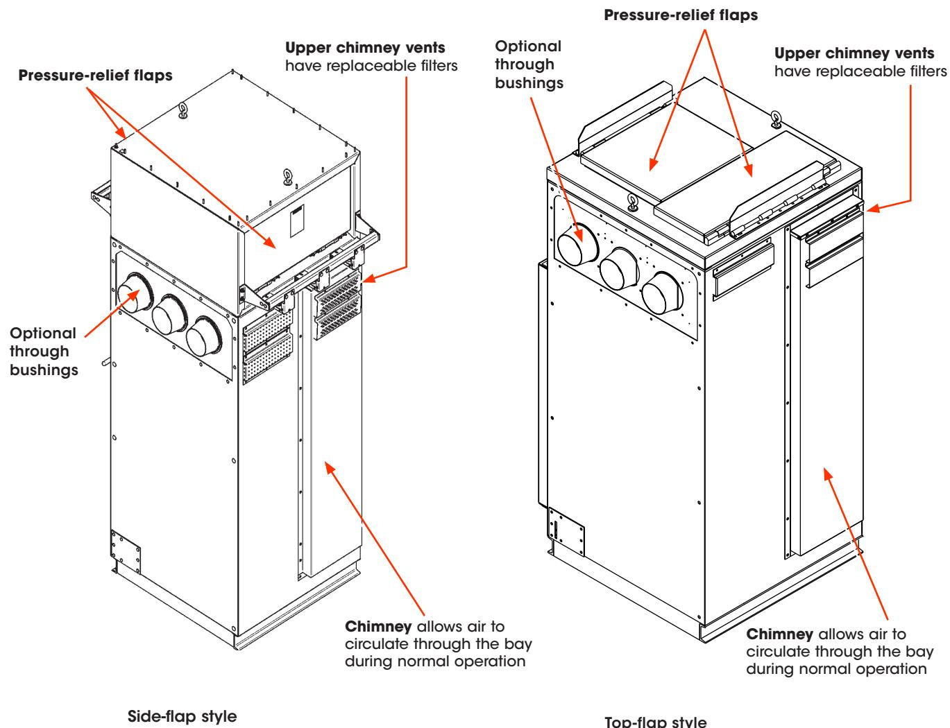
Figure 2. Rear view of arc-resistant S&C Metal-Enclosed Switchgear rated 15 kV, illustrating the rear chimney vent.
