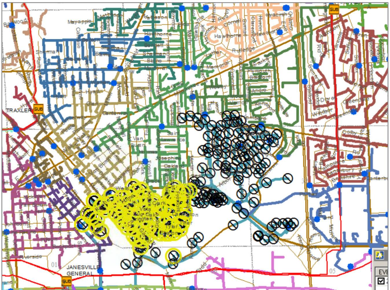
*An outage map showing Janesville customers out of power (in yellow) and where IntelliRupter fault interrupters restored power (noted in black).*
