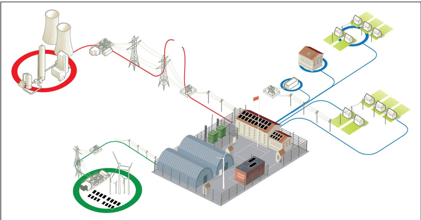
**"Quasi" microgrids serve loads with critical processes that depend on uninterrupted energy to operate. Local generation is used as a backup in case of a loss of the centralized utility source.**
